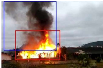
Sample detection: Red box for fire. Blue box for smoke.
